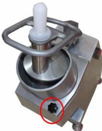
Using the knob, loosen the saftey catch by turning it counter-clockwise.
