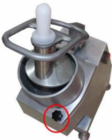
Using the knob, loosen the safety catch by turning it counter-clockwise.
